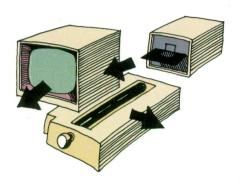
Although almost all computer attachments can be classified as either input or output devices, the disk drive is an input and output device—an I/O unit, in computer jargon. With a keyboard and monitor, plus this I/O device, you and your computer can communicate freely.
